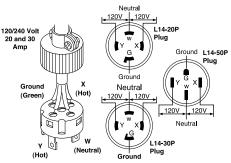
Figure 15 - Cord and Plug Configurations
